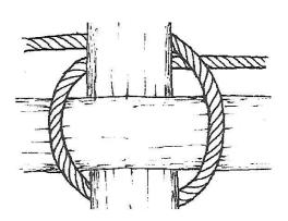
The Mark III is the same as the Mark II but a clove hitch is tied around the up right spar when starting the lashing.
