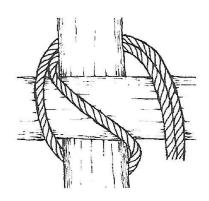
The MarkII Japanese Square Lashing is tied by looping the center of the rope of the upright spar and than forming the wrapping turns by taking the ends of the rope in opposite directions.
