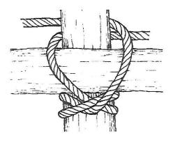
The Mark III is the most secure of the three Japanese square lashings because the clove hitch helps to prevent the lashing from shifting along the vertical spar.
